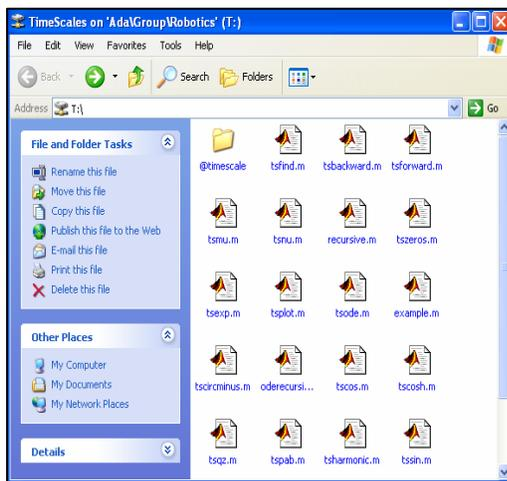
Once MatLab is opened, open the **tstoolbox** folder to access the time scale functions and operators.
